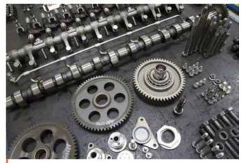
Some engine components requiring heat treatment
